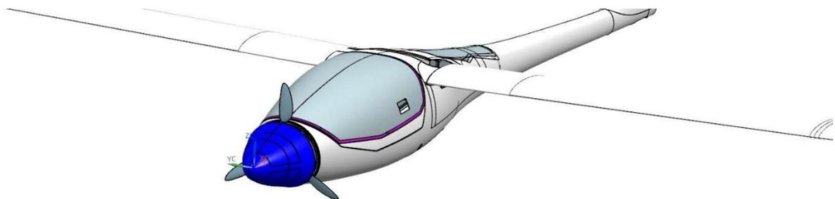
Foldable 3-blade propeller with a diameter of 1.45 m
