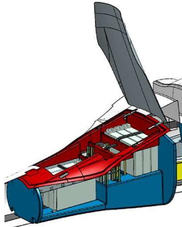
Two packages of 54 kg each with 400 V, each consisting of 3 modules of 18 kg each
