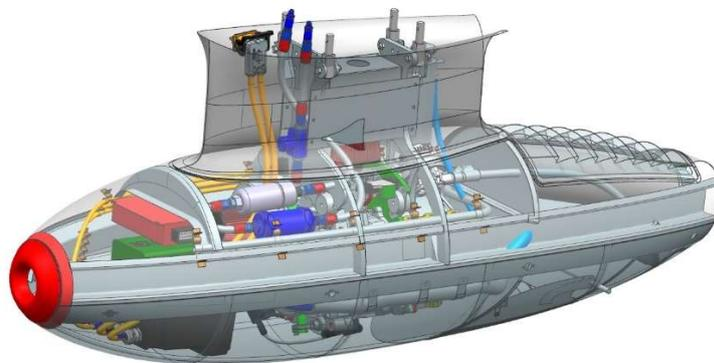
Electric generator system with 30 - 45 kW engine power
