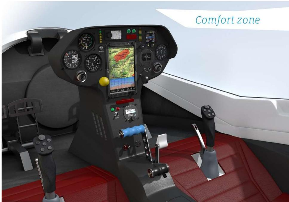
Often the ergonomics in the cockpit are considered for comfort. But it is also an active element of security. Pilots in a suitable environment make fewer mistakes. Thus, the cockpit is designed for pilots from 1.6 to 2.0 m and offers the appropriate panoramic view for each size. The minimum payload of 70 kg and the maximum of 200 kg allows almost every combination of two pilots to comply with legal regulations.
