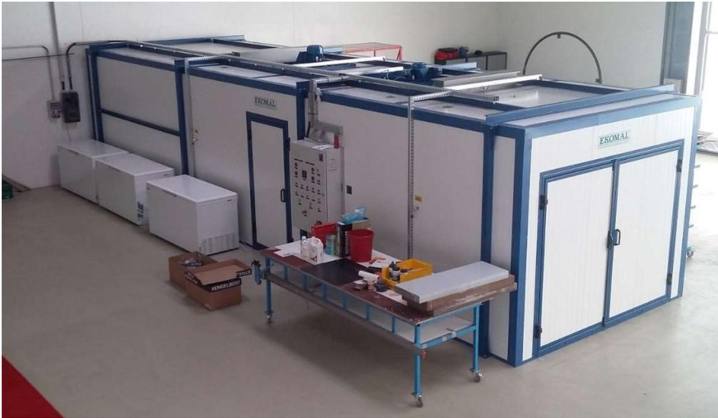
Three freezers with the prepeg raw material in front of the curing oven of 11 m length
