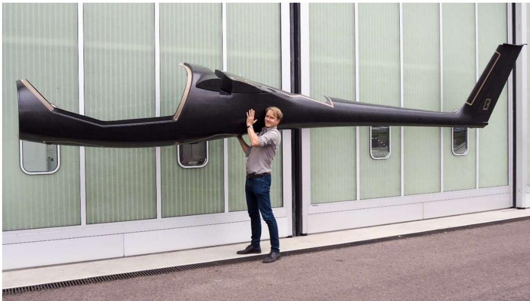
Goal achieved: 25% weight reduction compared to wet laminate and previous designs. One side of the fuselage constructed in prepeg, including reinforcement parts and integrated
