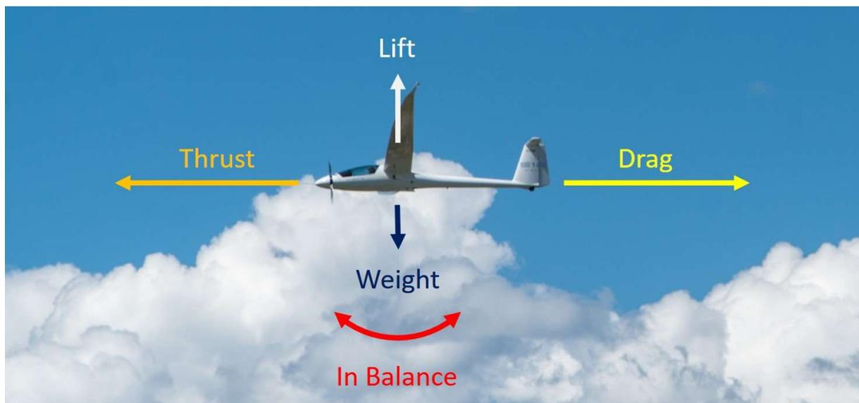
Force chart on the example of an S12 in powered flight
