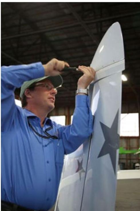
**Morgan Sandercock installing rudder cap complete with wide-angle camera**
